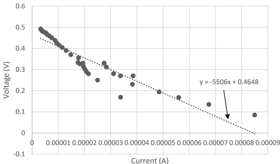
Figure 5. Current-Voltage plot for the MFC used for calculating the internal resistance.
