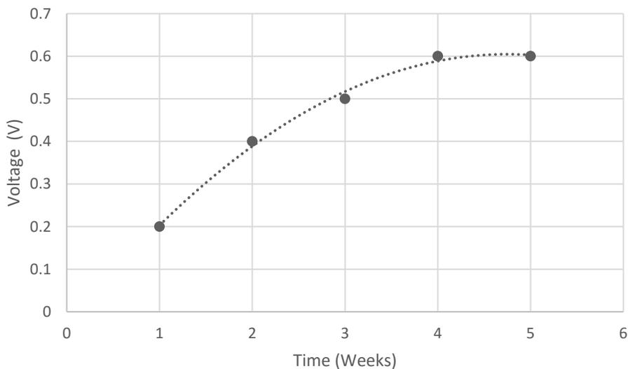
Figure 1. Development of the open circuit voltage of the MFC over a month.
