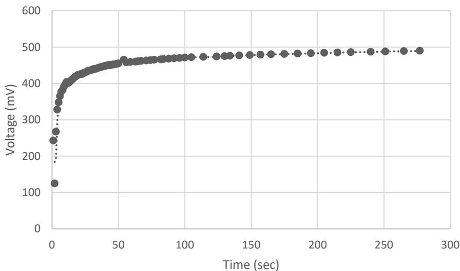
Figure 2. Time required for the MFC to achieve maximum open circuit voltage.
