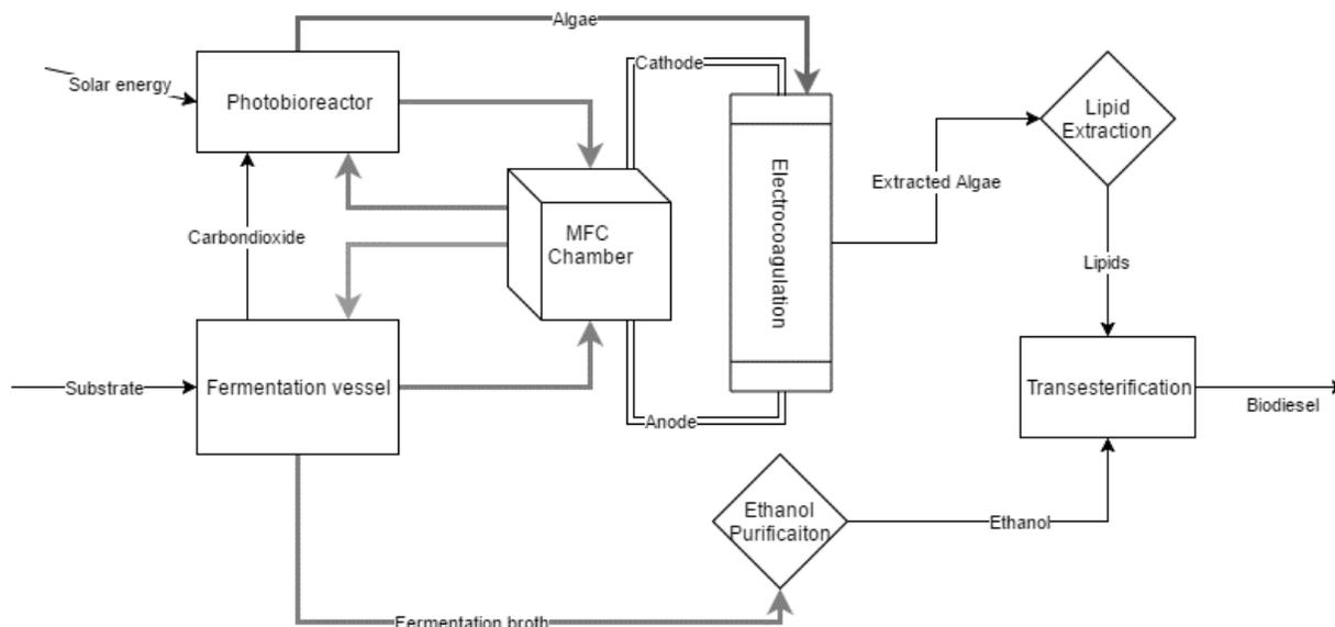
Figure 7. Flow diagram of the proposed combined algal growth and fermentation system along with electrocoagulation.
