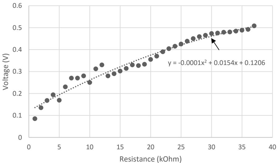
Figure 4. Voltage response of the MFC with change in the external resistance.
