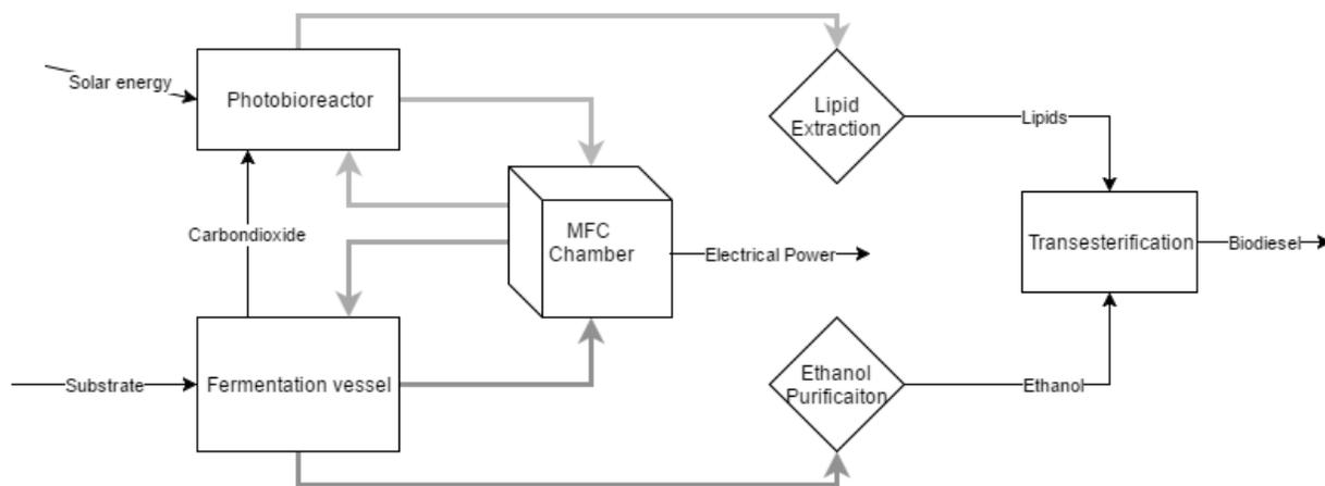
Figure 6. Flow diagram of the proposed combined algal growth and fermentation system.
