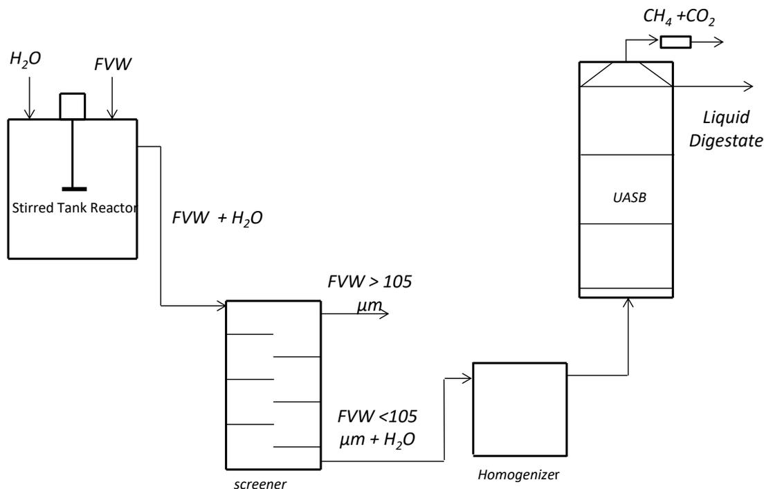
Figure 1. Two-stage anaerobic system.
