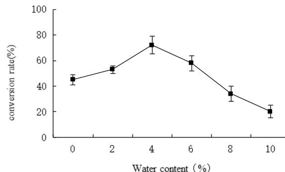
Figure 11. Effect of water contents on biodiesel conversion.
