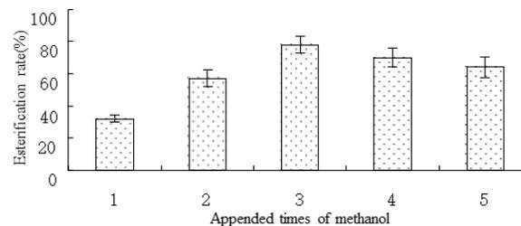
**Figure 8.** Effect of appended times of methanol on esterification rate of artificial sour oil.
