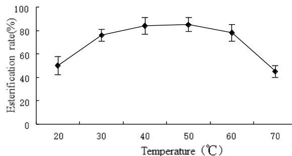
**Figure 6.** Effect of reaction temperature on esterification rate of artificial sour oil.
