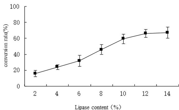
Figure 10. Effect of lipase contents on biodiesel conversion.
