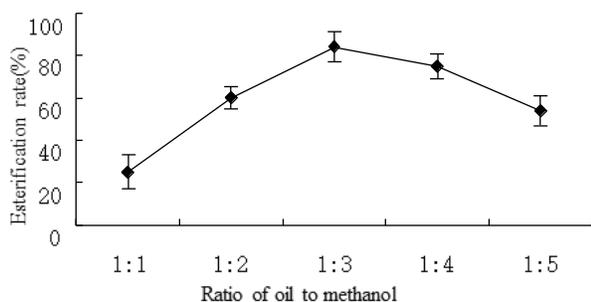
**Figure 5.** Effect of molar ratio of methanol to oil on esterification rate of artificial sour oil.
