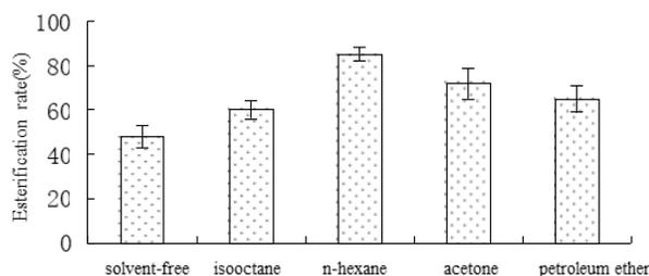
**Figure 3.** Effect of different solvent on esterification rate of artificial sour oil.
