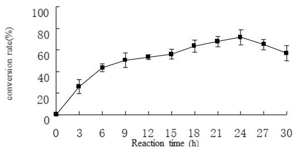
**Figure 13.** Effect of reaction time on biodiesel conversion.
