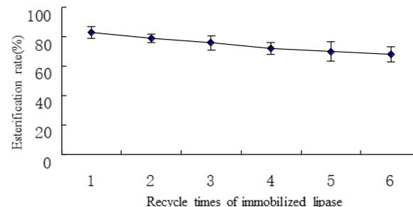
**Figure 9.** Effect of recycle times of immobilized lipase on esterification rate of artificial sour oil.
