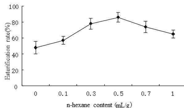
**Figure 4.** Effect of n-hexane contents on esterification rate of artificial sour oil.
