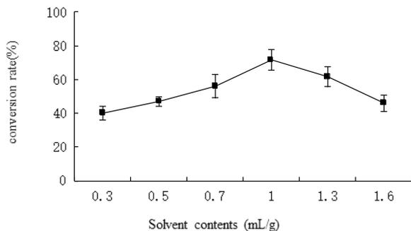
**Figure 12.** Effect of organic solvent contents on biodiesel conversion.
