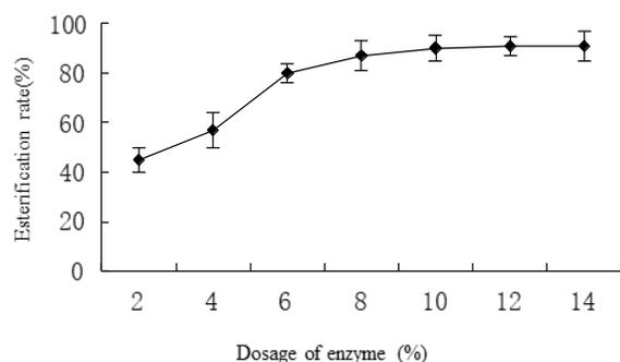
**Figure 1.** Effect of lipase dosages on esterification rate of artificial sour oil.
