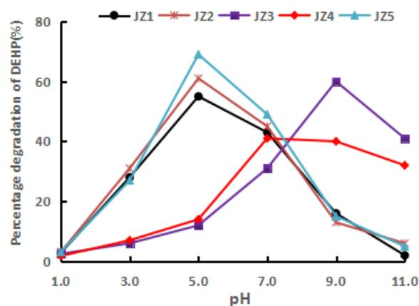
Figure 1. Effect of pH on degradation of DEHP.
