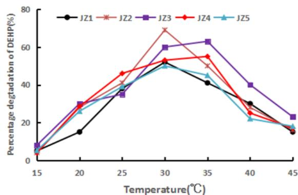
Figure 2. Effect of temperature on degradation of DEHP.
