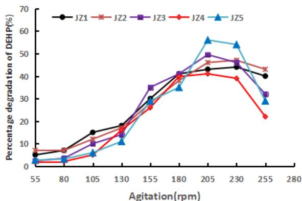
Figure 3. Effect of agitation on degradation of DEHP.
