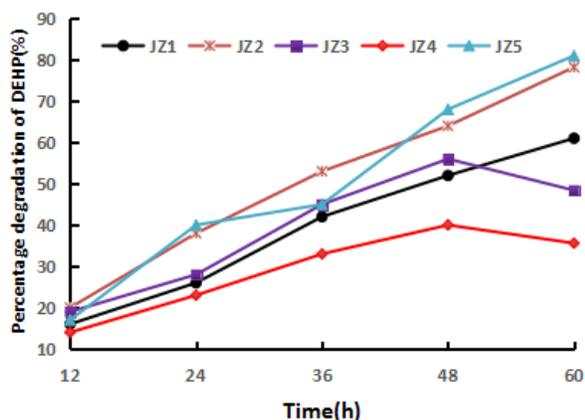
Figure 4. Effect of time on degradation of DEHP.
