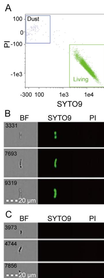
Figure 2. Live and dead *S. pasteurii* based on multispectral imaging flow cytometry.
