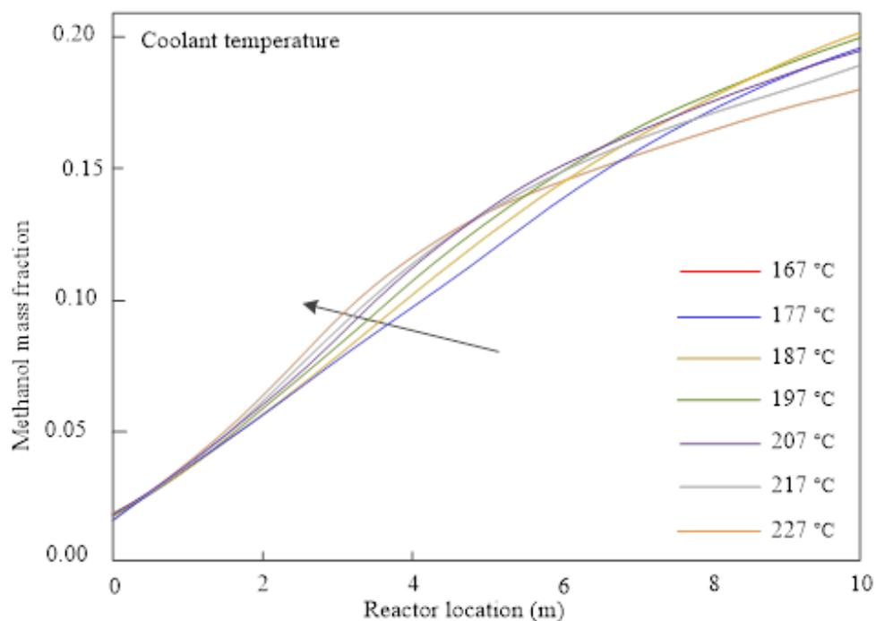
**Figure 4.** Effects of coolant temperature on temperature distribution curve (A) and methanol mass fraction distribution curve (B) in reactor.
