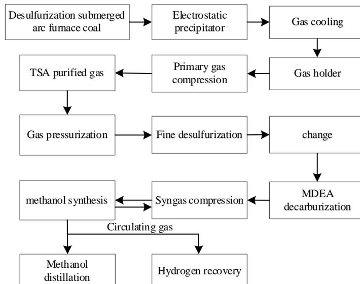
Figure 3. Process flow chart of methanol production from coal catalysis.
