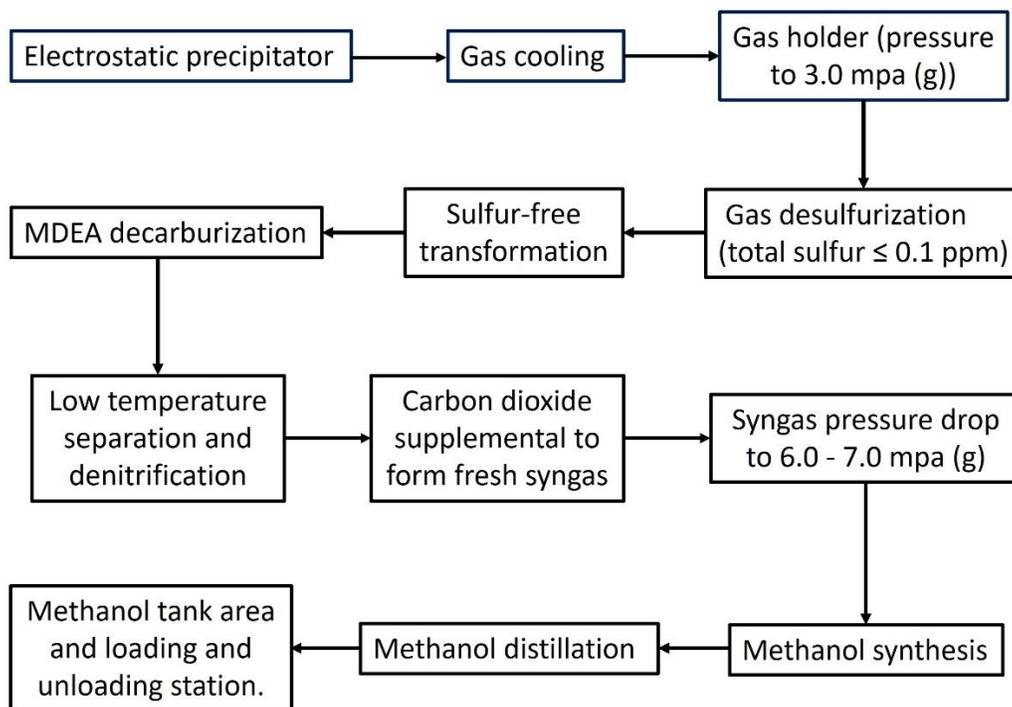
**Figure 1.** The scheme for methanol synthesis process.
