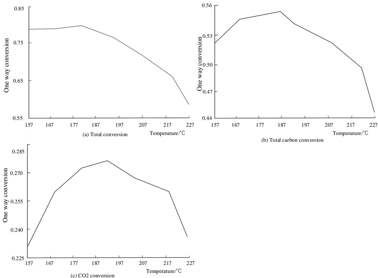
Figure 5. Effects of coolant temperature on one-way conversion.
