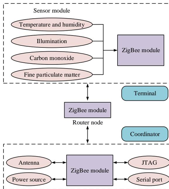
Figure 1. Structure of each module in ZigBee network.
